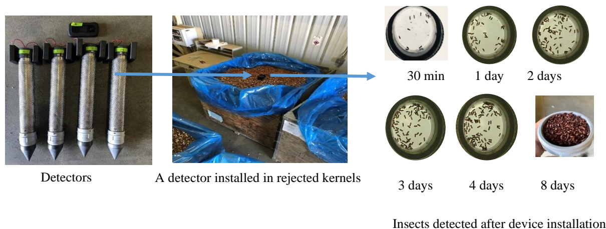
Figure 6. Detectors and insects detected after installation in rejected almond kernels
