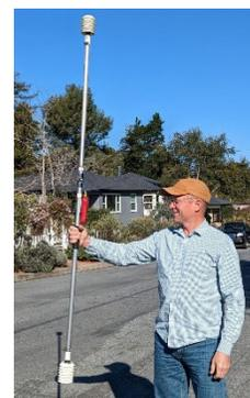
Inexpensive tool that can measure near-ground temperature inversion conditions in real time.
