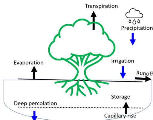
Figure 1: Evapotranspiration process and soil water balance
