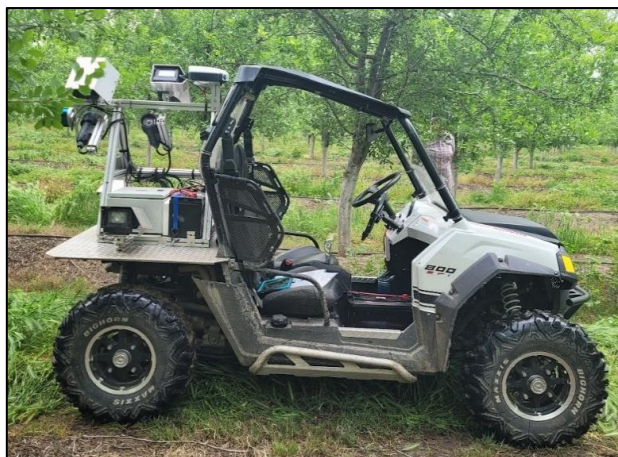
Figure 1. Dropcopter's Green Atlas Cartographer in a prune orchard.
