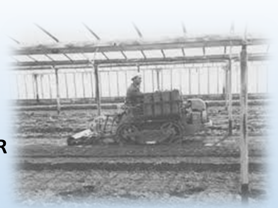
Fumigating glasshouses with chloropicrin using an injection rig mounted on a Ransomes MG6 tractor 1960.
