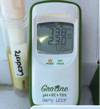
**Figure 2**: Measuring Electrical Conductivity with a portable EC meter.
