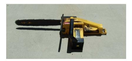
A gasoline-powered chain saw is shown below. Such saws are available with varying engine sizes and bar lengths, and always have an automatic chain oiler. They are dangerous but useful if operated carefully. Chain saws are not simple tools that can be operated intuitively (with no training or reference to their instruction manual). In recent years, chain saws have anti-kickback features that increase operator safety. Appropriate safety clothing should be worn.
