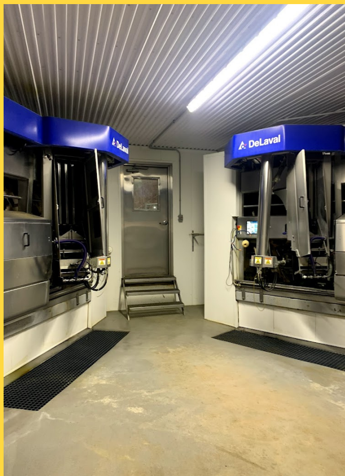
FIG 4. BOOTH-SHAPED DESIGN OF AMS UNITS
