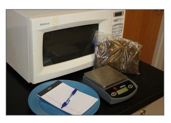
1. Equipment needed: microwave, preferably with a turn table; microwave safe plate (not paper); gram scale accurate to at least 1.0 gram; representative sample; note pad & pen; a well ventilated space.
