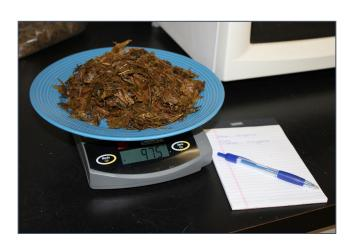
3. Place about 100 grams of a representative sample on the plate. Weigh and record as sample + plate.
