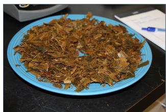
4. Arrange the sample so that it is spread evenly across the container and not more than 1.5 inches high. Leave a small depression in the center of the container (should resemble a donut).
