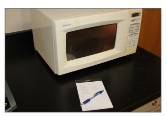
Mix the forage and arrange so that it is again evenly distributed and resembles a donut. Return the container to the microwave and heat for an additional 30 seconds if almost dry, or 1 minute if still wet.
