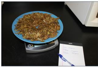
6. Open the door and allow any steam to dissipate. Remove the container, reweigh it, and record this weight.
