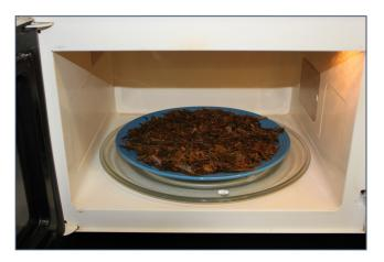
Place the sample container in the microwave. For wet forages (silages), start by heating the material for 2 minutes on high. All microwaves are different, so some of this will be trial and error with your specific model.
