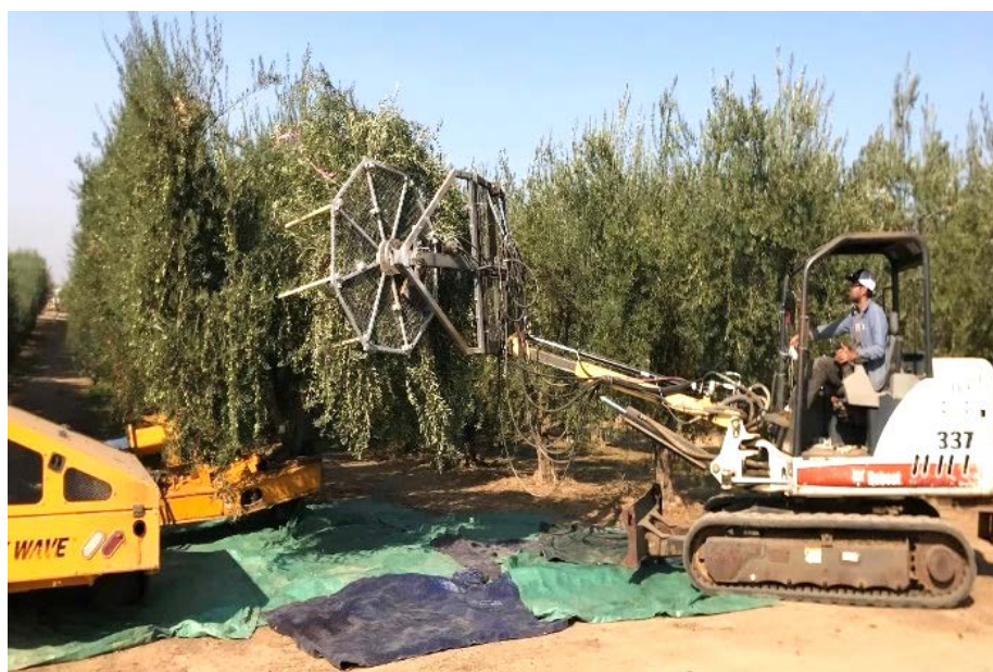
Figure 11. Trunk and canopy shaker simultaneously shaking an olive tree.
