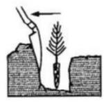
Straighten back of hole and insert seedling at proper depth. The top of the root plug should be at least 1/2 to 1 inch below the soil line as long as the foilage will not be buried.
