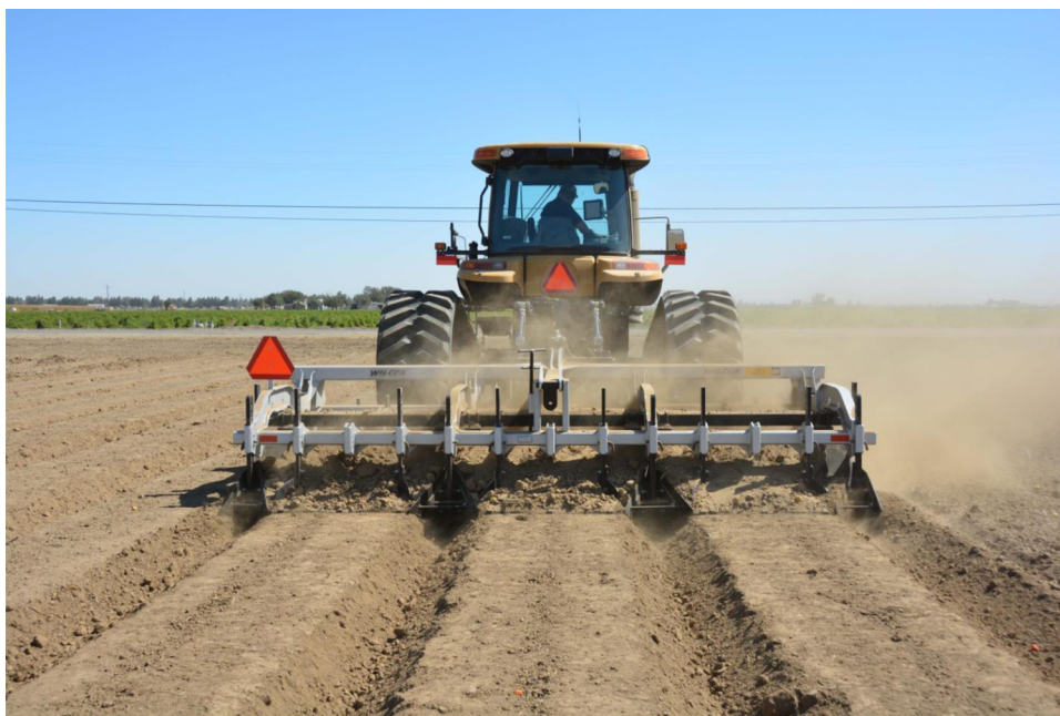
Photo 4. Reworking beds with the minimum tillage, pass-combining Performer implement (Wilcox Agriproducts, Walnut Grove, CA), 2014, (Photo: A.Wilcox).
