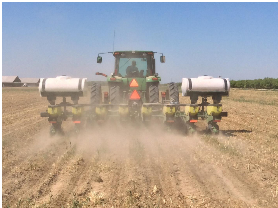
Photo 6. Strip-tillage and seeding operations conducted by California Ag Solutions, (Madera, CA) with Central Valley dairy silage farmers who are interested in learning about strip-tillage, 2014, (Photo: M. Bottens).
