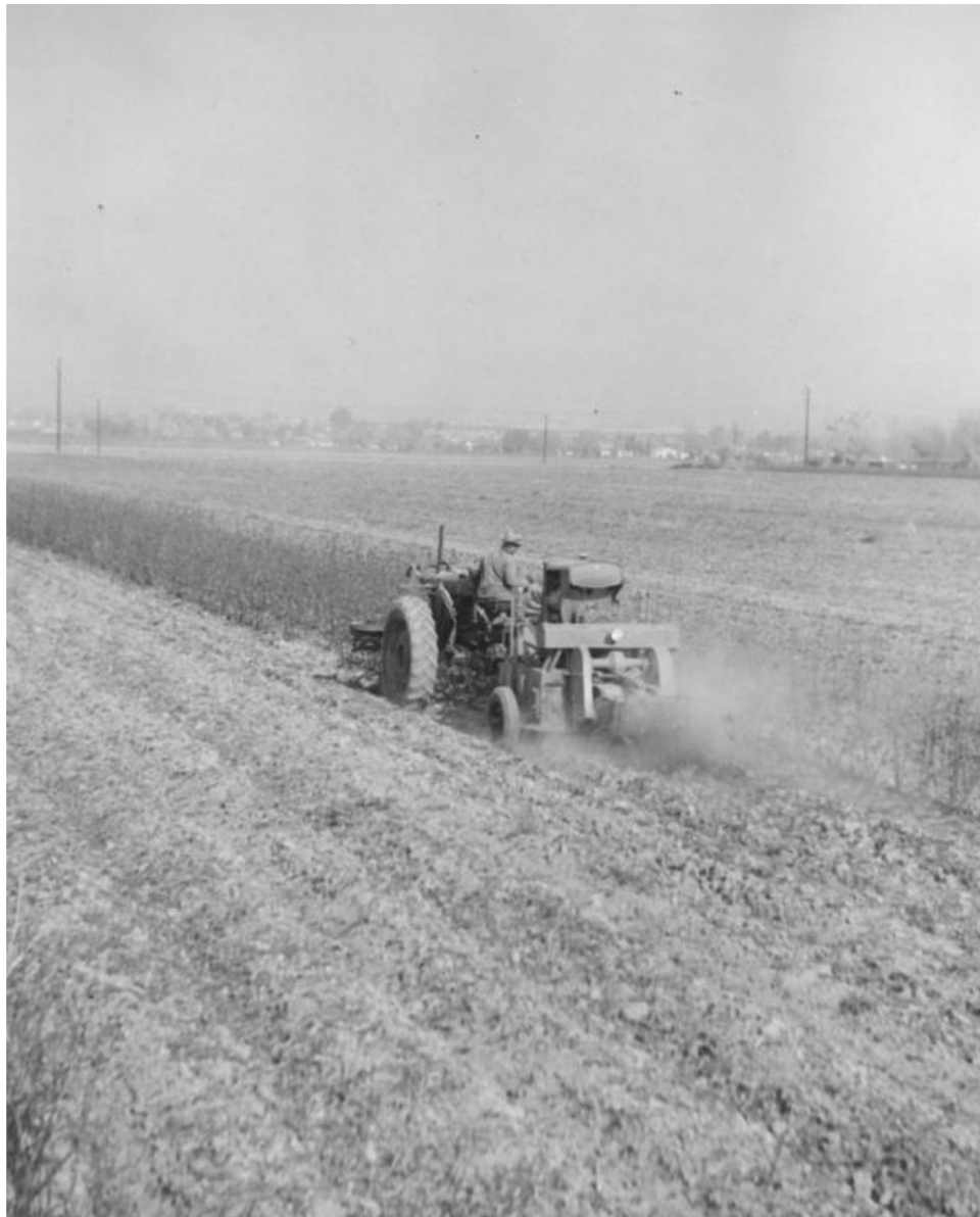
Photo 1. Shredder-Bedder (Interstate Mfg., Bakersfield, CA), a one-pass cotton postharvest rebidding implement designed and developed by Al Rouzi, 1958 (Photo: A. Rouzi).
