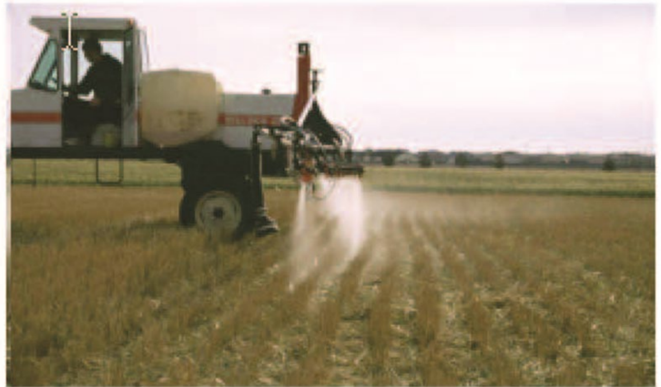
Figure 3. Air induction nozzles at 70 psi. (Wolf)
