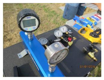
**Pressure gauge testing is available!** If you would like your sprayer gauge tested against a certified accurate gauge, please remove your gauge from your sprayer and label it by writing your name and phone number on a piece of masking tape and tape it to the back of the gauge. Drop off your gauge at Kautz Farms between 10 a.m.- 2 p.m. on Feb. 19-the day before the actual training. Your gauge will be returned at the end of class with the accuracy information kept confidential.
