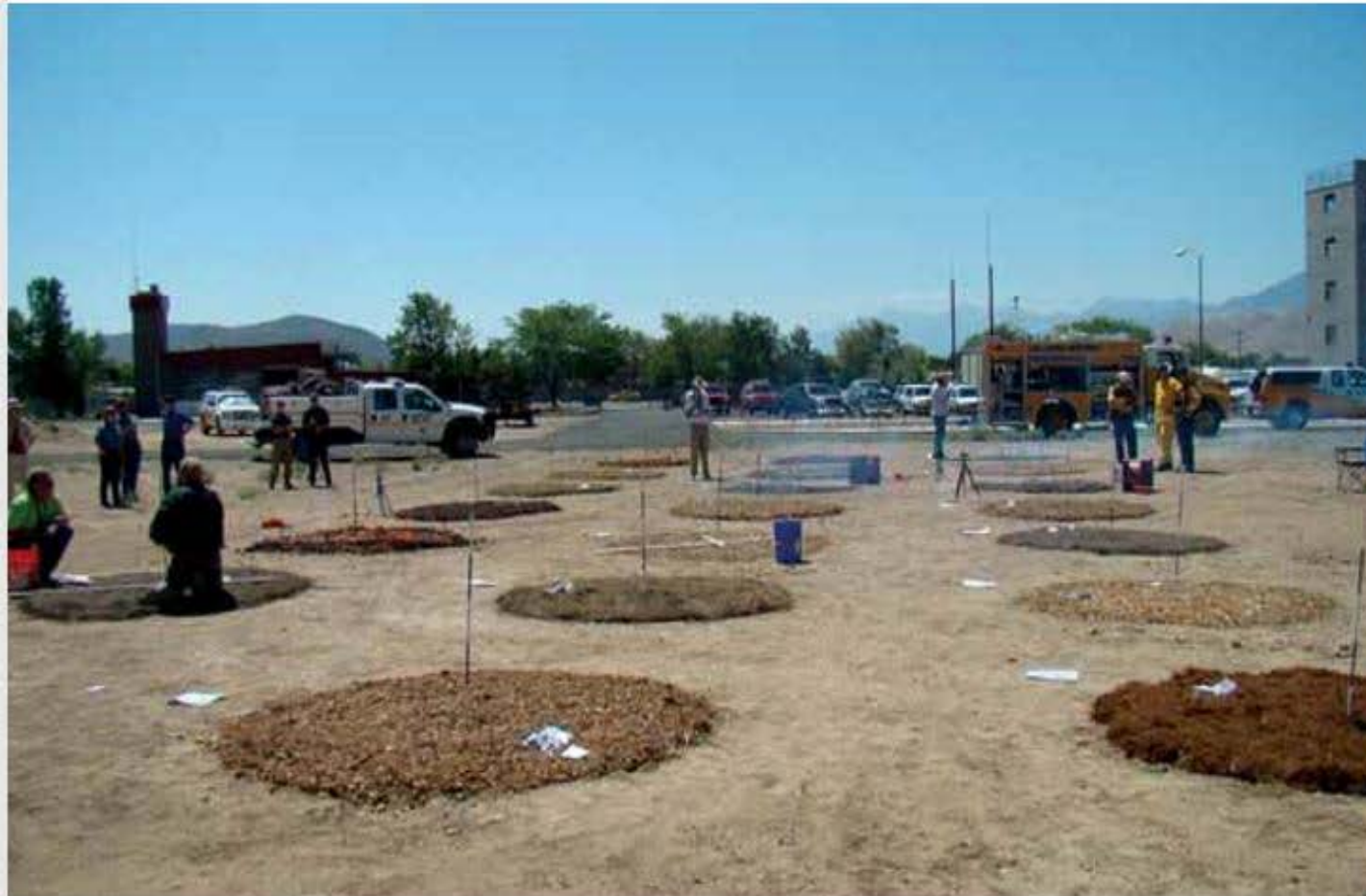
◀ Figure 2. The eight different mulch treatments were replicated three times and randomly positioned within the plot layout on May 28, 2008. After being exposed to the elements for over 2½ months, they were ignited on Aug. 14, 2008.
