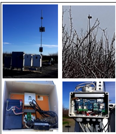
Figure 7. Parts of a telemetry system. Cell tower and gateway next to pump controls (top left), gateway connection to internet (bottom left), orchard cell tower connected to sensors in the field (top right); and node connection to field sensors (bottom right).
