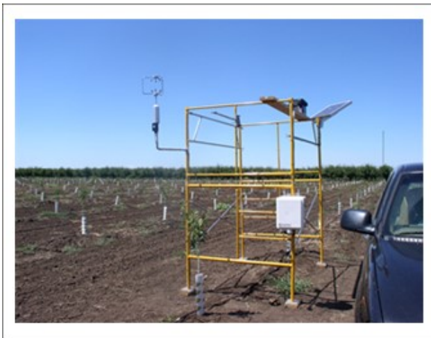
Figure 1. Field instrumentation used in newly planted prune orchard to measure crop ET.
