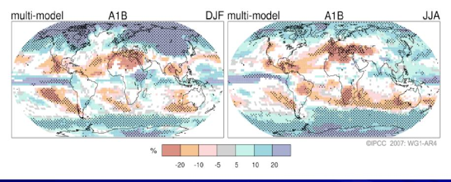
Relative changes in precipitation (by percent) for the period 2090-2099, relative to 1980-1999. Values are multi-model averages based on the SRES based on the A1B scenario for December to February (left) and June to August (right). White areas are where 66% of the models agree on the sign of the change and stippled areas are where more than 90% of the models agree on the sign of the change.
