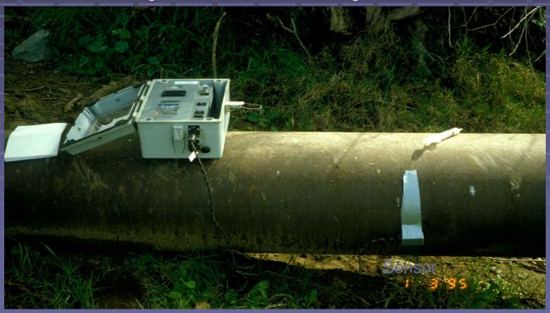
pipe cross-sectional area X water velocity = Flow rate
