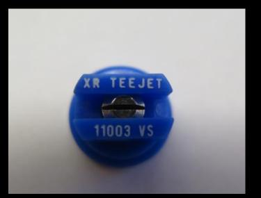
This XR (extended range) flat fan nozzle is a 11003. It should deliver 0.3 gallons per minute at 40 psi with a spray angle of 110°. The VS stands for "visiflow", the nozzle body material (visiflow plastic).
