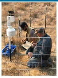
Matthew Shapero and Dr. Royce Larsen working to install a digital rain gauge at a forage plot on the Gaviota Coast. Precipitation totals are monitored at each plot and are coupled with forage production data to understand how the timing and amount of rain changes the amount and composition of forage on rangelands.
