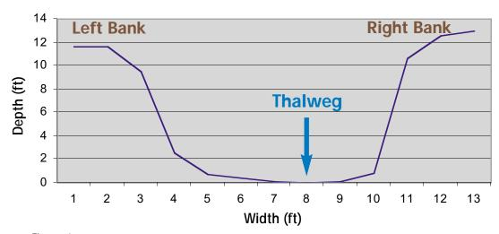
Figure 4. Measurements taken in the field can be converted to a graphical representation of the channel morphology. Labeling the banks and thalweg (the deepest part of the channel) helps keep the graph in perspective.
