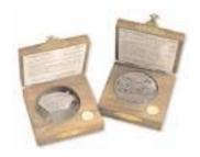
Figure 6. Spherical densiometers are used to measure canopy cover.
