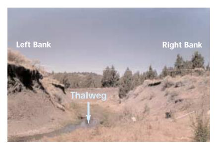
Figure 5. Actual site described graphically in Figure 4. The tape can be seen stretched across the stream, and left and right banks as well as thalweg are highlighted for reference.
