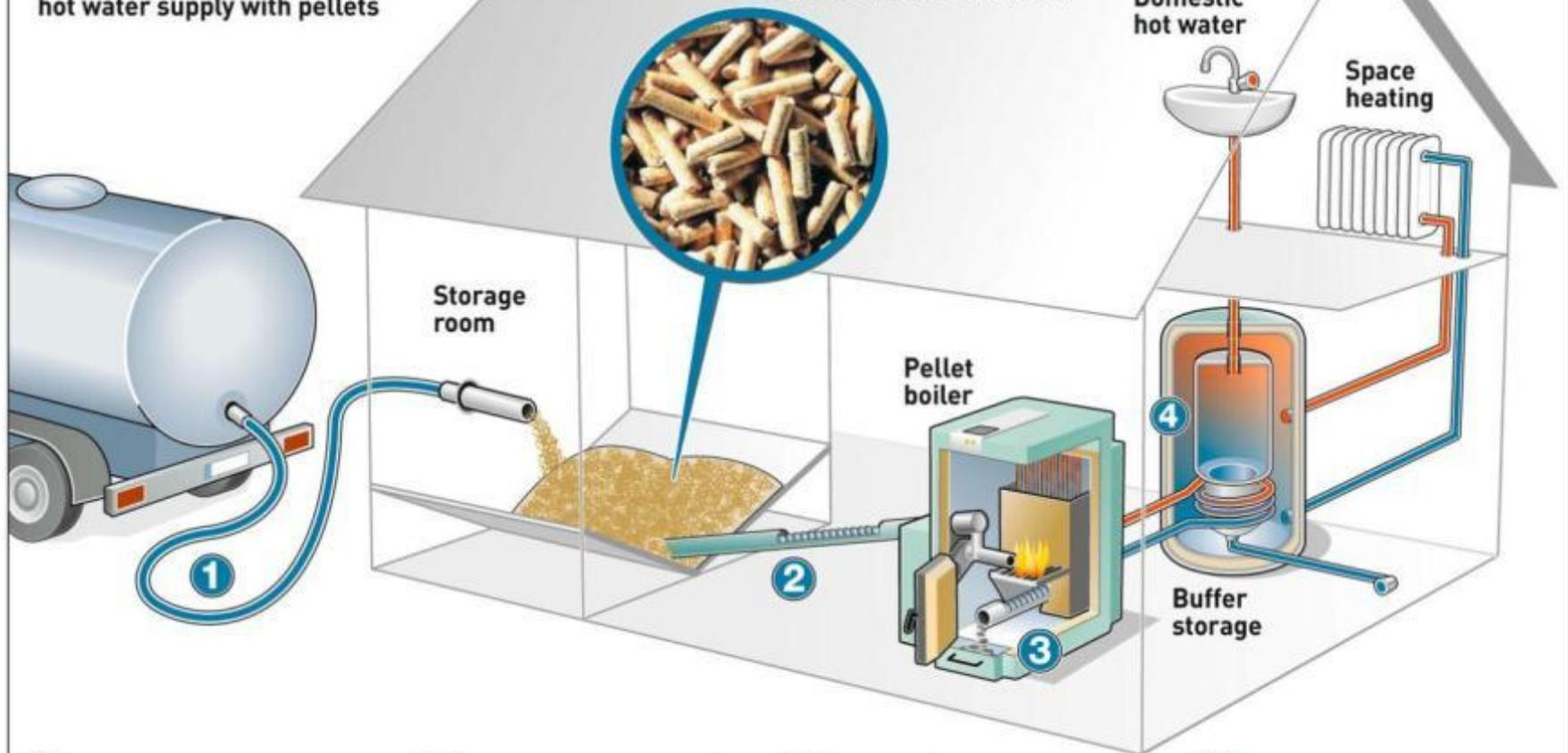
**1** Once or twice a year the pellets are delivered by a silo tanker. A loaded storage room of 4.5 m<sup>2</sup> is enough to keep a single-family house warm for one year.
