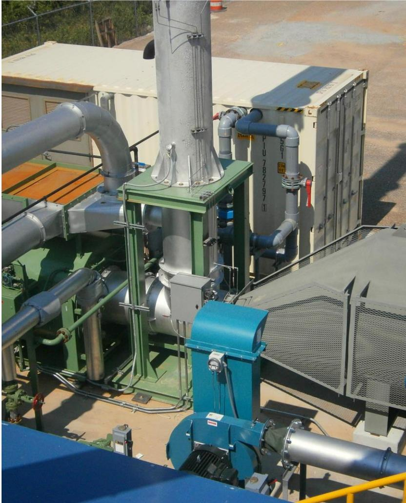
**1. Fuel Gas is Combusted** in a thermal oxidizer to cleanly produce heat
