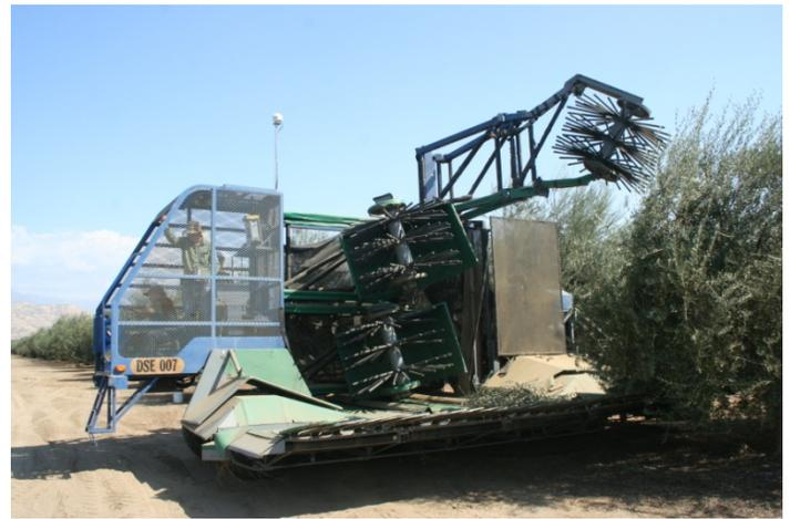
Fig. 1. 2008 version of the canopy contact head olive harvester originally modified from wine grape harvesters in 1996. This harvester can be used as one of a pair, or as a single that does both sides of the tree. The head is mounted on a catch frame that conveys the fruit back to a field bin.
