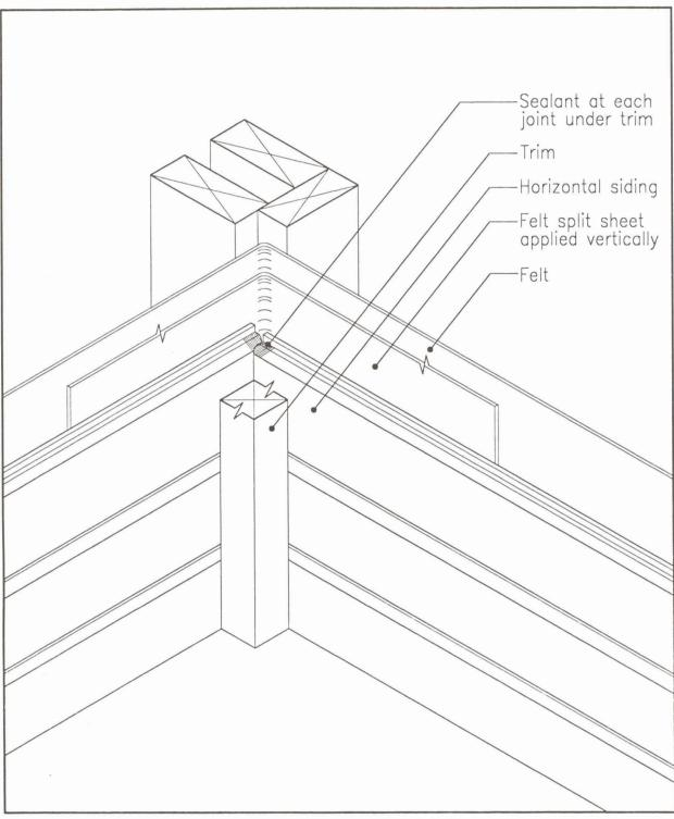
LUMBER VERTICAL JOINT INTERNAL CORNER DETAIL
