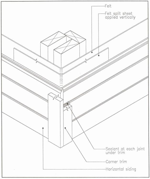
LUMBER VERTICAL JOINT EXTERNAL CORNER DETAIL
