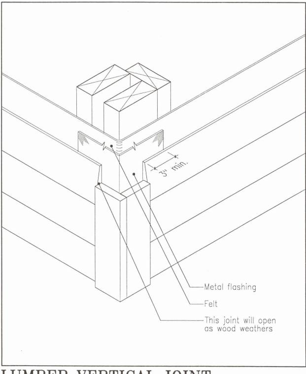
LUMBER VERTICAL JOINT EXTERNAL CORNER DETAIL
