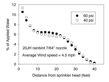
Figure 1. Average distribution of water from a rainbird 20JH sprinkler head with a 7/64 inch diameter nozzle at pressures of 60 and 40 psi and average wind speeds of 4.5 mph.
