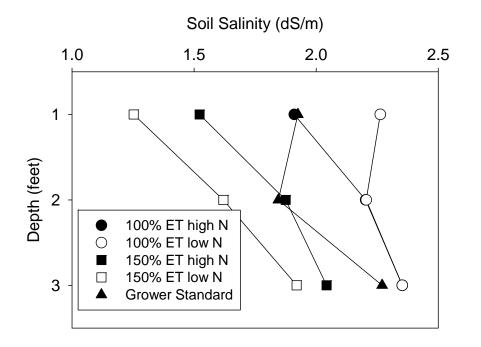
Figure 9. Irrigation and N fertilizer treatment effects on soil salinity measured after harvest in iceberg (north county trial [1]).
