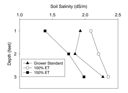
Figure 1. Irrigation treatment effects on soil salinity measured after harvest in iceberg (north county trial [1]). Means for the 100% and 150% ET treatments represent the average of the high and low N treatments.
