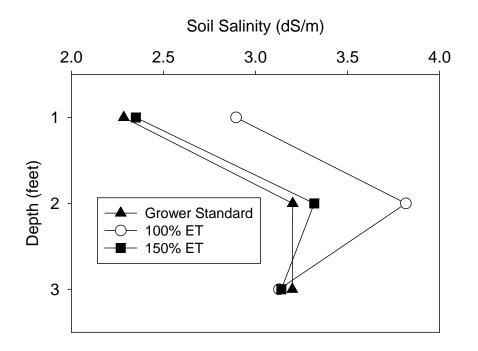
Figure 2. Irrigation treatment effects on soil salinity measured after harvest in romaine (south county trial [2]). Means for the 100% and 150% ET treatments represent the average of the high and low N treatments.
