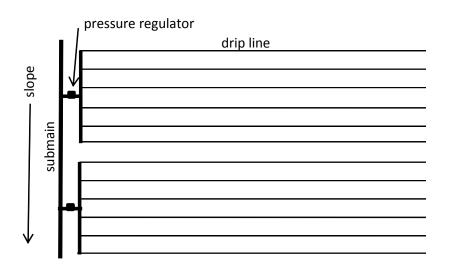
Figure 3. Use of preset pressure regulators on the submain to regulate pressure in groups of drip lines located at similar elevations.
