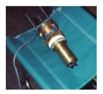
Figure 4. Turbine flowmeter. Photo: Lawrence J. Schwankl.
