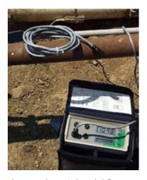
Figure 3. Ultrasonic (Doppler) flowmeter. Photo: Lawrence J. Schwankl.
