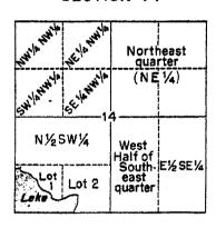
Figure 1. Generalized diagram of land division within the U.S. System of Rectangular Surveys.
