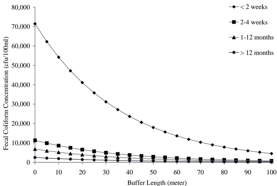
**Figure 40:** Results for pasture management from data-driven model of fecal coliform concentration as influenced by the amount of time since manure was spread and the length of vegetated buffer strip. The storm size (i.e. 24-hour cumulative precipitation) was also a significant factor in the model and held constant at 0.5 inches in this graph (Lewis et al. 2010).
