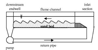
FIG. 1. Schematic diagram of the recirculating flume used for *C. parvum* oocyst deposition experiments.
