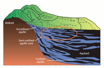
Figure 4. Unconfined, semi-confined, and confined aquifers in a typical California alluvial basin. Dark-colored sediments indicate fine-grained clay or predominantly clay materials (*aquitard*). Light-colored materials indicate coarser-grained aquifer materials.
