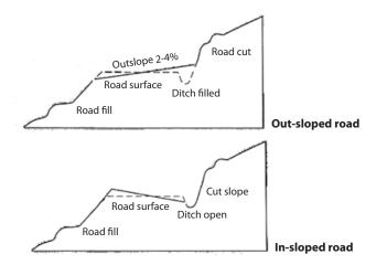
Figure 8. Out-sloped and in-sloped road cross-sections. Source: Adapted from Weaver and Hagens 1994, p. 47.
