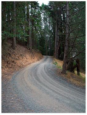
**Figure 10.** There is a gentle rolling dip in the middle of this picture of an out-sloped road. *Photo:* Richard Harris.
