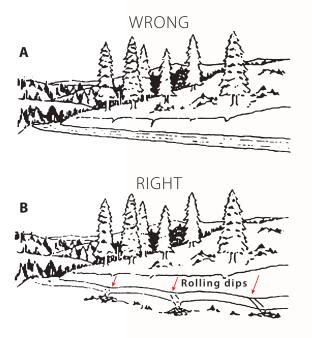
**Figure 7.** A: A road surface that is not properly drained will concentrate surface water runoff that will eventually erode the road bed. B: Out-sloping the road and installing rolling dips to drain runoff minimizes water concentration and erosion. *Source:* Adapted from Weaver and Hagens 1994, p. 47.
