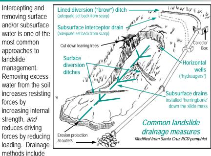
surface diversions, roof runoff management, subsurface drains, grading to reduce infiltration through cracks, and others. Covering the slide with plastic to reduce infiltration is discouraged; installation and maintenance can be difficult, soil moisture is retained, and the plastic may obscure incipient failure.
