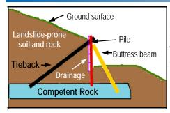
Structural retention systems increase resisting forces by providing lateral support. Measures include retaining walls, pilings, tieback anchors, and anchored gabions. These measures may be used in combination with soil reinforcement measures that increase internal strength. Ensuring proper drainage is a critical
