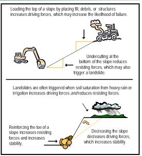
building pads. Natural events or land use activities may not be identified as a triggering mechanism, but may contribute to failure by lowering the slope's threshold for failure, making it more likely that failure will occur in response to some triggering event.
