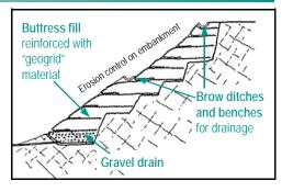
may be reinforced with geomembranes or geosynthetics. Ensuring proper drainage is a critical component of design, and larger buttress fills in particular require evaluation and design by a qualified engineer.
